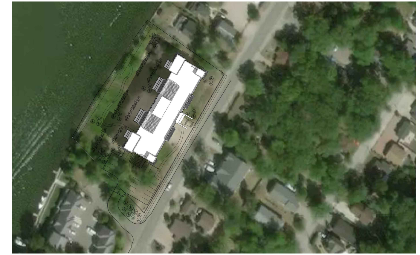
10:00 MAR/SEPT 21 MORNING SHADOWING HAS NO AFFECT ON NEIGHBOURING PROPERTIES
