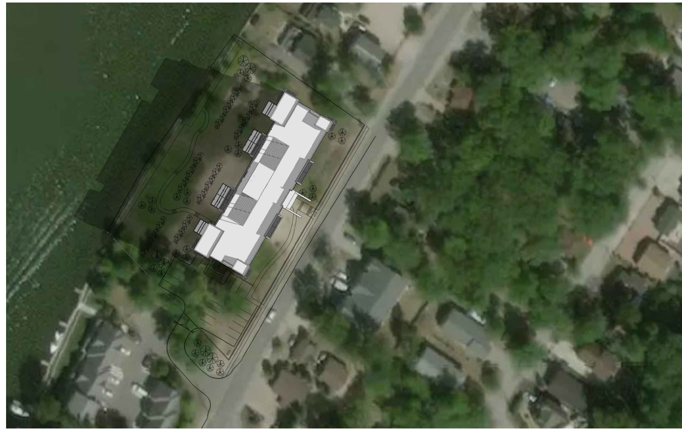
8:00 MAR/SEPT 21 MORNING SHADOWING HAS NO AFFECT ON NEIGHBOURING PROPERTIES
