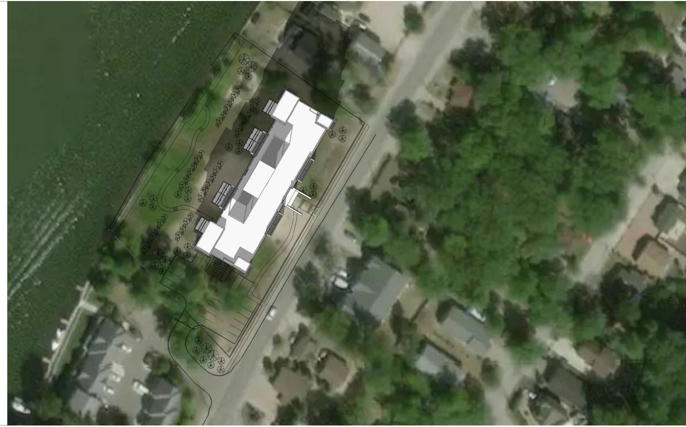
1:00 DEC 21 AFTERNOON SHADOWING AFFECTS 2 PROPERTIES TO NORTH, BUILDINGS PARTIALLY SHADED
