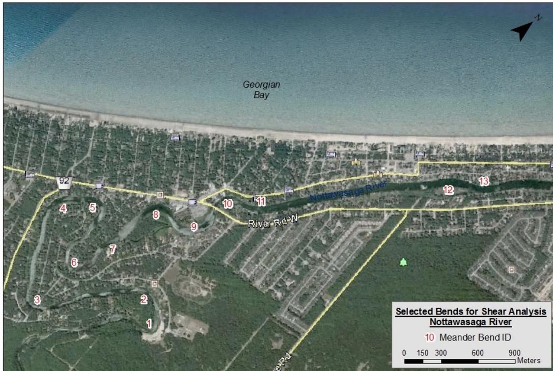
**Figure 6: Bend Locations for Shear Analysis.**
